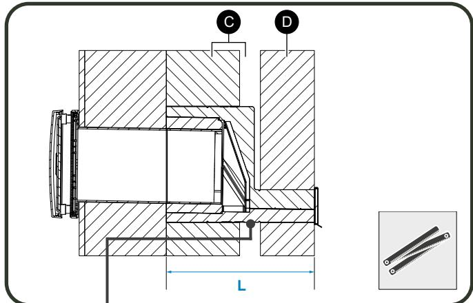
Option 2: Dämmsystem WDVS (insulation)
